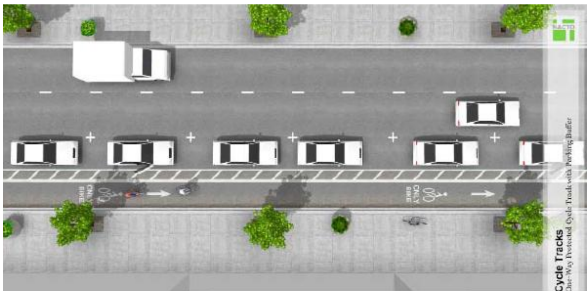
One-way cycle track with on-street parking as the buffer from the motor vehicle travel lanes. Note the use of “parking T’s” to designate the on-street parking spaces. (Source: NACTO Urban Bikeway Design Guide)
