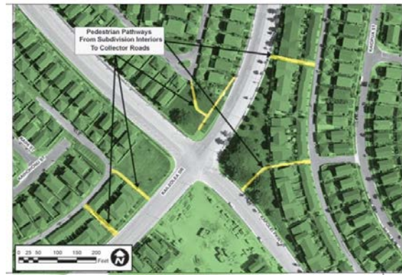
Pedestrian networks can be re-established by opening noise walls and connecting new sidewalks. (Credit: PB Americas, EWA Connection Study , May 2009)
