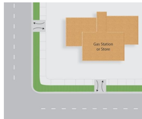
Reconstructed corner with fewer, narrower driveways (Credit: Michele Weisbart)
